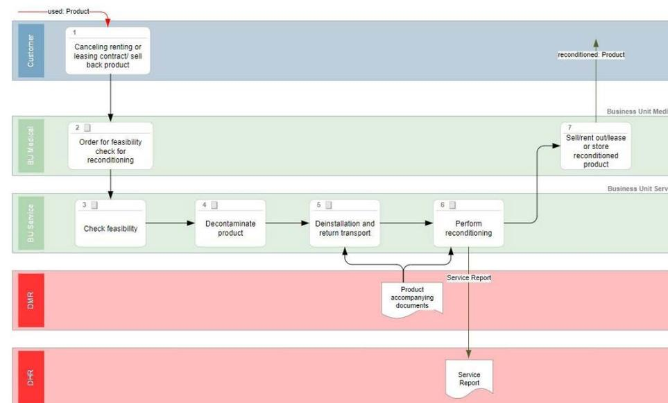
Figure 8 – Equipment Reconditioning Process
