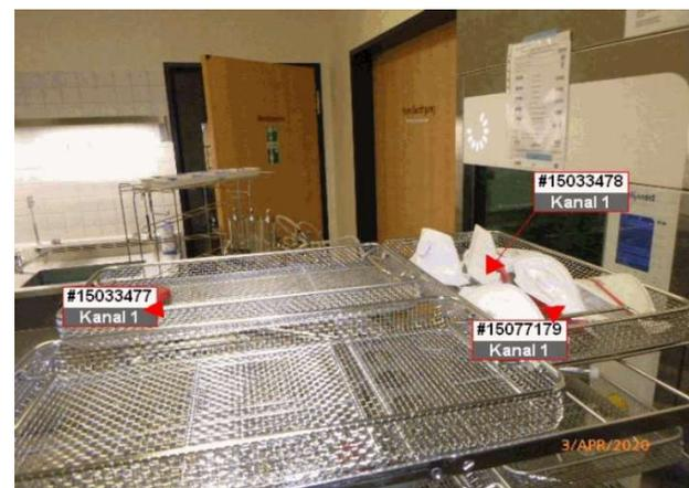
Picture 8: Four level rack with FFP2 masks and temperature loggers on various levels
